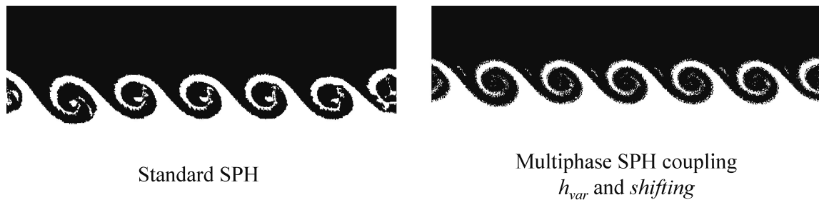
Fig. 7. Results of the Kelvin-Helmholtz instability test.
