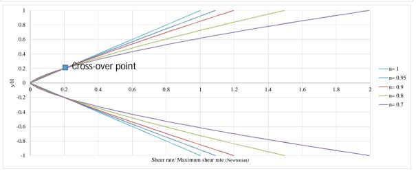
$0 > \frac{y}{H} > 0.2 \rightarrow$  Shear rate of Newtonian fluid > Shear rate of non - Newtonian 0.2 < y/H < 1  $\rightarrow$  Shear rate of Newtonian fluid < Shear rate of non - Newtonian
