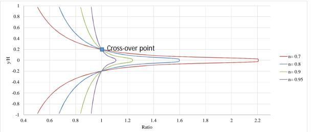
$0 > y/H > 0.2 \rightarrow Viscosity$  of Newtonian fluid < Viscosity of non - Newtonian
